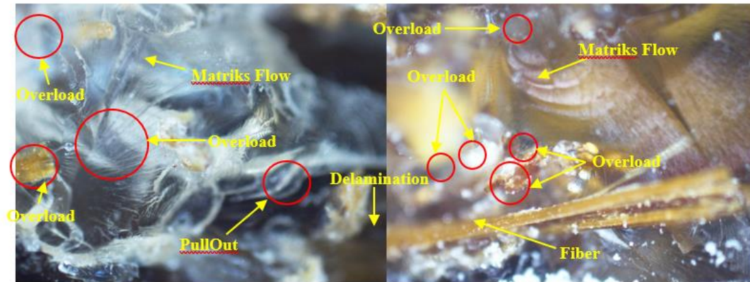
Figure 9. Micro photo of bending & tensile fractures volume fraction variation 30 % Fiber 5x magnification.
