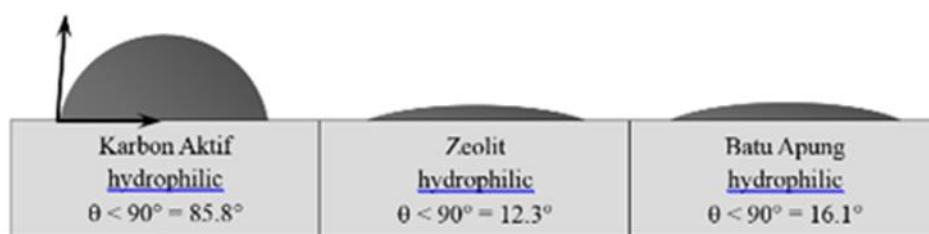
Figure 4. The value of the contact angle on each surface of the material.
