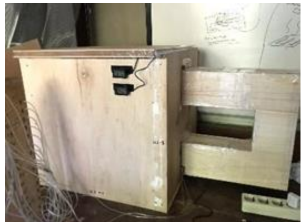
Figure 3. Air conditioning test room. Notes: (1) The test room is built using plywood with dimensions of 50cm x 50cm; (2) The test chamber channel is 40cm x 8cm; (3) The computer fan measures 8cm x 8cm; (4) The test material container or packed bed.
